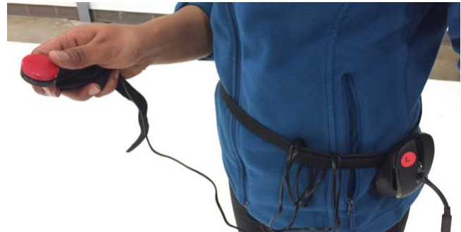
Figure 4. Researcher demonstrating the kick button controller prototype based on a modified Bluetooth wireless mouse.
