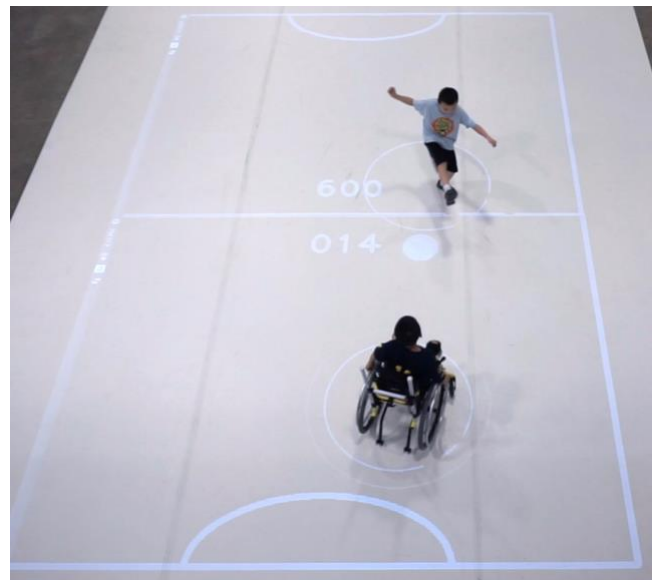
Figure 1. Two children competing on iGYM 's interactive floor. The projected circles around their bodies can be expanded – through body movement or with a kick button – to manipulate a virtual target into the opponent's goal. The scores are displayed at the center of the playground.
